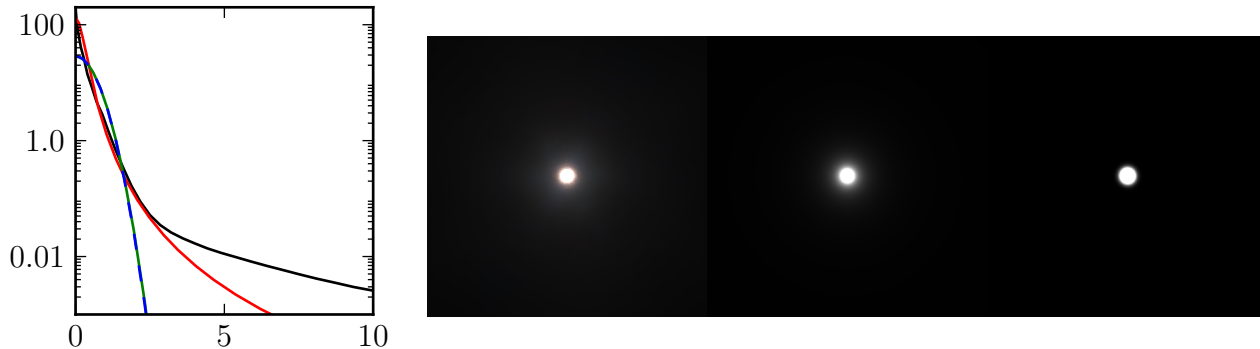
Figure 9: Several specular distributions fit to MERL chrome. Left: log-scale plots of specular peak vs \theta_h (degrees); black = chrome, red = GGX ( \alpha = 0.006 ), green = Beckmann ( m = 0.013 ), blue = Blinn Phong ( n = 12000 ). Right: (clipped) point light responses from chrome, GGX, and Beckmann.
