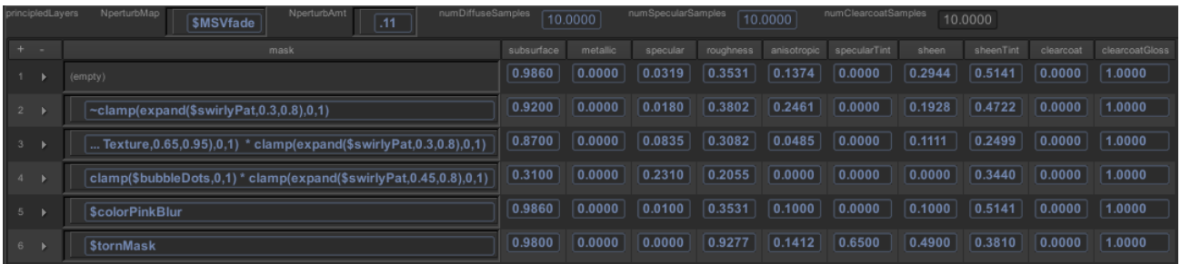
Figure 20: A screenshot of our shader editor showing material layers. The variables in the mask expressions refer to spatially varying shader modules, typically texture maps.
